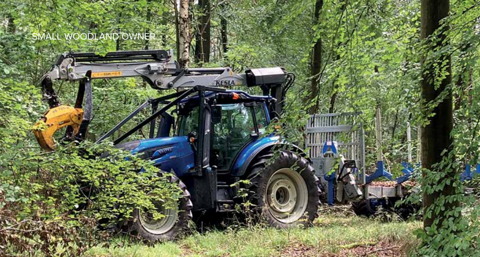
Small tractor and trailer fitted with grab and hoist to become a forwarder. Good for gathering firewood piles on easily worked sites.
