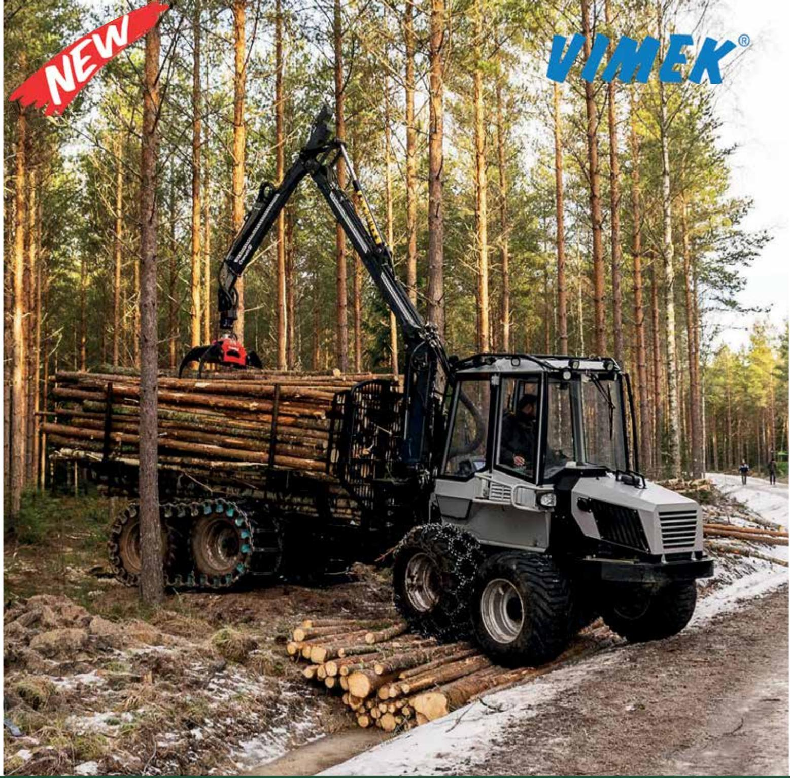
Vimek has developed a brand new machine for the Next Generation project. The new forwarder has a 7.5 tonne carrying capacity and is powered by a 75hp, turbocharged Caterpillar engine and Bosch Rexroth transmission. This forwarder has a brand new larger cab with better visibility, better sound insulation and LED lights around the entire machine. A new Cranab crane has also been developed to be the perfect match for this forwarder with a reach of 6.7 meters.
