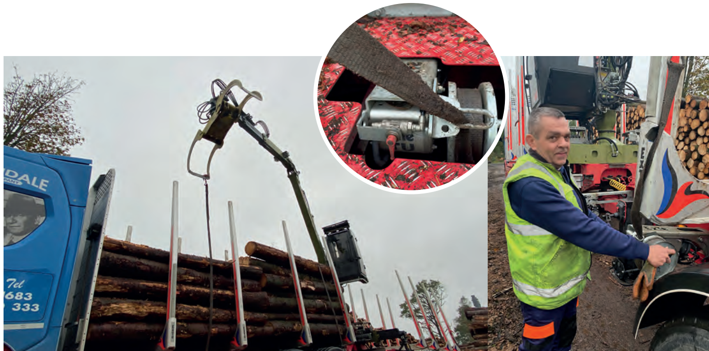
Left to right: The crane grab raising the strap over the loaded timber. The strap is tensioned via a drum winch. Brian Greggan of Annandale Transport demonstrates the TU Auto Tensioner
