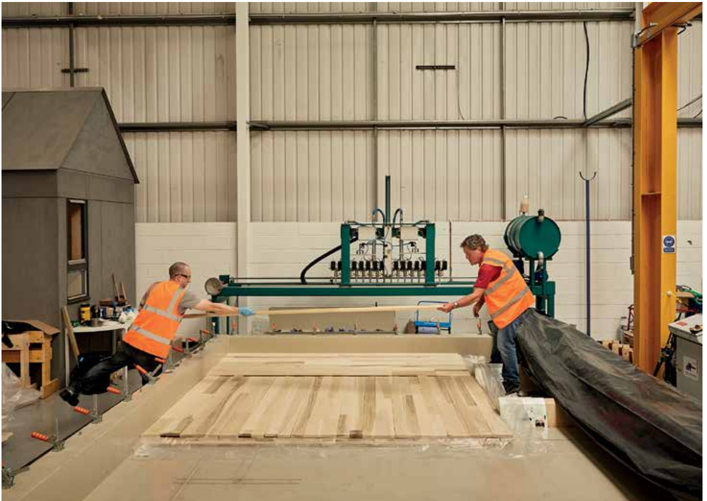
Construction Scotland Innovation Centre - vacuum press for CLT manufacture
