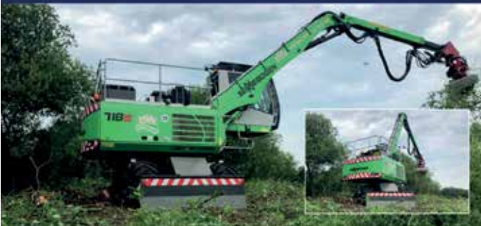
Upto 15m reach with a selection of attachments the Sennobogen 718e is ideal for ash dieback on tracks and highways
