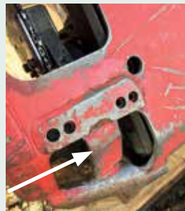
Saw box type of chainshot protective device
