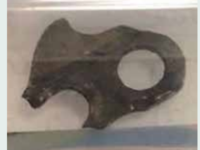
Above: Chainshot involved in a near fatal accident that became embedded in the injured party having passed through the protective screen.
