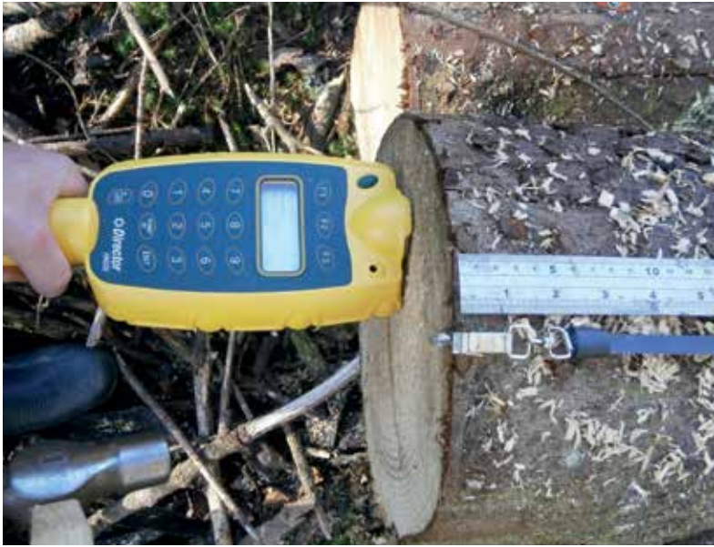
Resonance assessment used to estimate the stiffness of the first three 3.1m long logs from each felled tree in the Farigaig trial. © Forest Research
