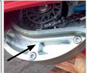
Chainshot protective device closely fitted around drive sprocket
