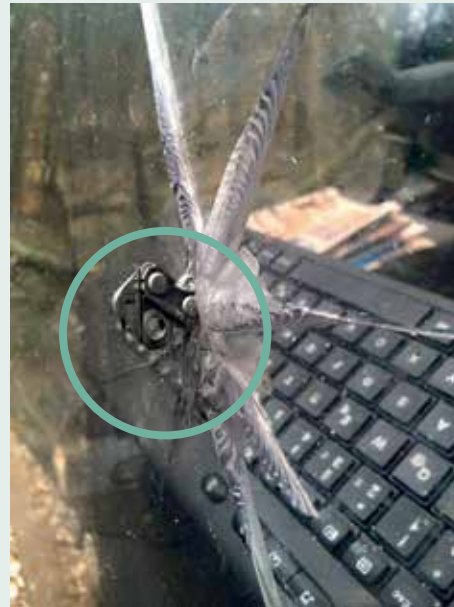
Below: Chainshot embedded in or having passed through the protective screen
