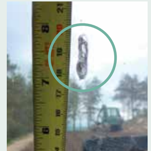
Above: Chainshot involved in a near fatal accident that became embedded in the injured party having passed through the protective screen.
