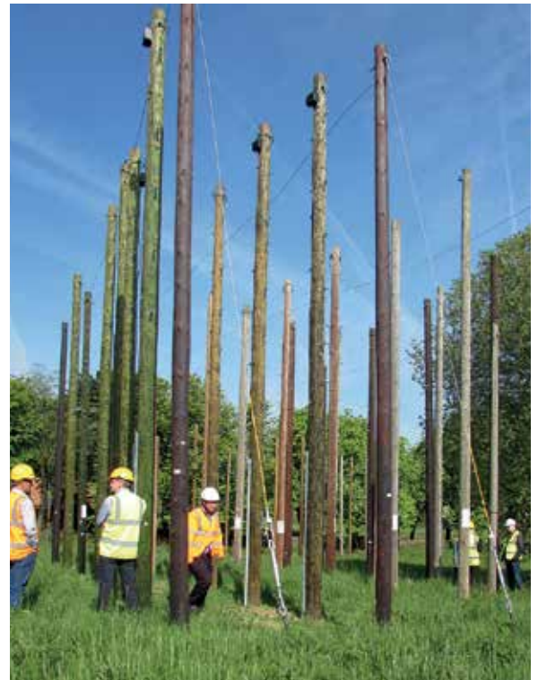
Field testing of modern and traditional preservative treatments for communication poles.
