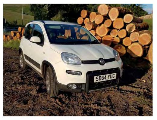
is automatically shifted to the rear wheels, in the same way as it would in a Discovery Sport or VW Tiguan. However the Panda 4x4 has a special button for calling up drive to all four wheels which you can engage before moving off, say on a slippery steep snow covered incline. It works very well and removes front wheel slippage while power is being shifted rearwards. Even BBC's Top Gear drove one to the top of a mountain beating Suzuki's Ignis, for what it's worth!
