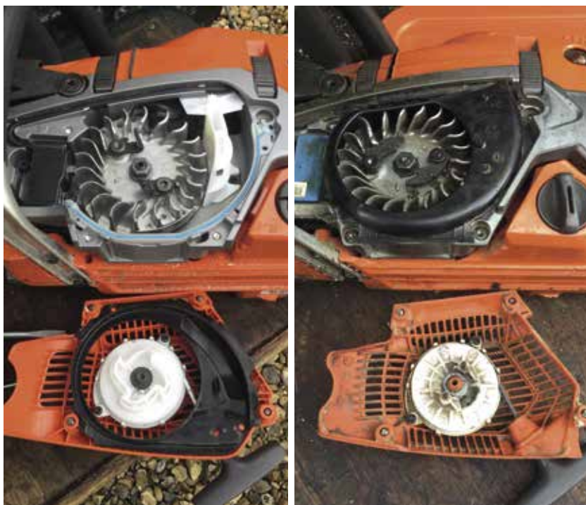
Mark 11 (left) starter and fly wheel layout - better organised and easier to clean than Mark 1 (right)
