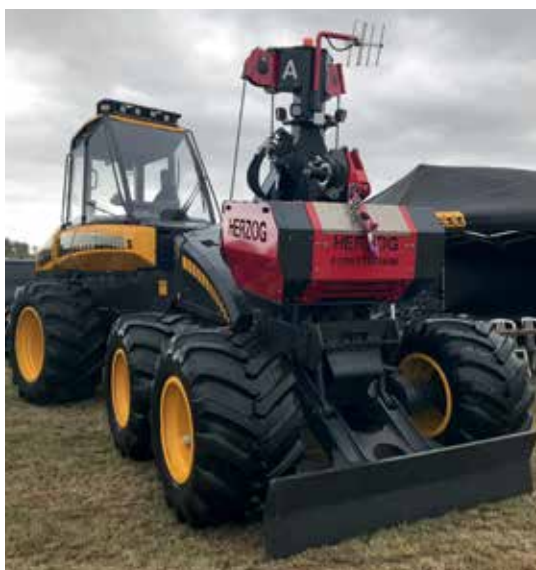
Ponsse Ergo with the Herzog Forsttechnik AG traction aid winch
