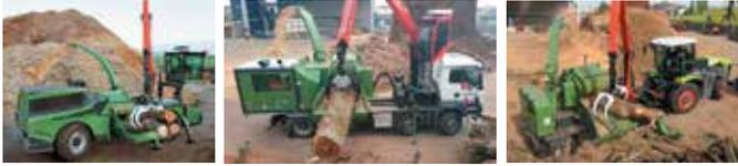
Wide range up to 400 m<sup>3</sup>/h, robust and large diameter CLOSED drum, customised cutting configurations, adjustable cutting depth, designed for easy feeding, hydraulic opening counterblade. *Options inc:* hydraulic fan, rubber belt discharge, sliding chassis, rotating platform
