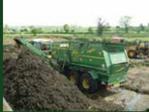
The Zago Eco Green Composter supplied by King Feeders UK offers a simple, reliable and economic means of green waste recycling. Because these machines operate at a very low noise and nuisance level, they are favoured by many local authorities for use in urban areas. They grind, mulch and mix bio-degradable products, from grass mowings, roots and soil to ten inch diameter tree loppings, pallets, waste paper etc.
