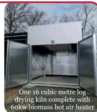
One 16 cubic metre log drying kiln complete with 60kw biomass hot air heater
