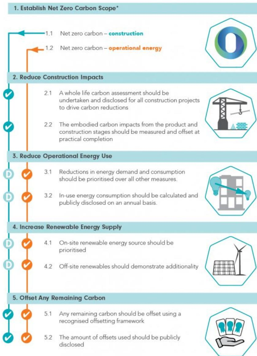
*Figure 1: The steps towards achieving net zero carbon for a built asset according to the UKGBC's definition. Source: Net zero carbon buildings: A framework definition (UKGBC, 2019).*
