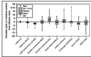
Figure 1 Measuring deviations from the reference value for the manual rapid moisture content determination systems
