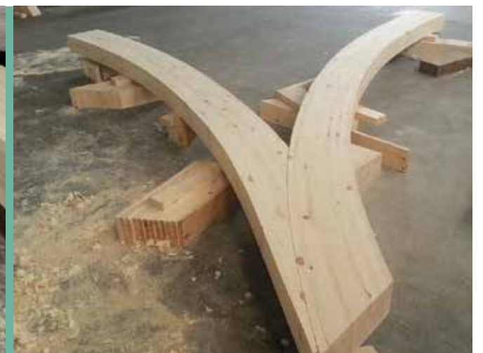
Left to right: Grand Designs on site filming manufacturing process at Buckland Timber, for a Channel 4 series; curved joint for Timber Kit Solutions; 1.75m radius curves Above: Robin Nicholson Top: Glulam portal frame structure for a church hall building
