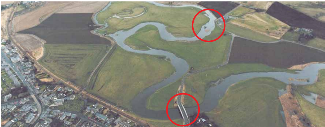
Figure 14: Bridge structure at risk of failing due to erosion from inappropriate location on an active river.
