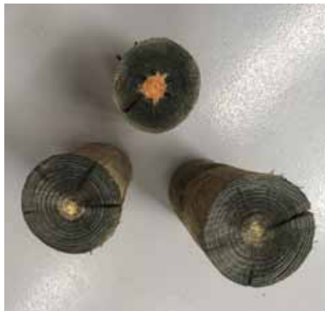
Right: Cross section samples of pine 30 yr dsl posts sprayed with copper reagent reveals the preservative penetration achieved without incising.
